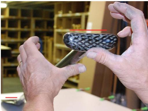
After firmly pressing the t-top into place, sight down the shaft to ensure that the t-top is parallel to the blade. Note the red lines in the photo.
