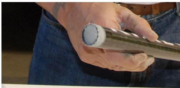
4. Use regular setting 2-part epoxy glue. **Make sure to use an adequate amount of glue to ensure a water-tight seal.** Failure to do so may cause water to leak into the shaft. For best results do not use a fast drying epoxy and do let it dry 24 hours before use.
