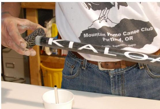
NOTE: The t-top is a snug fit, use good pressure and a twisting motion until it bottoms out. Bracing the blade on a padded or carpeted floor while pressing on the t-top is helpful.
