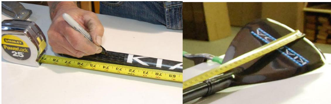
Measure from the tip of the blade, as shown. It is not necessary to adjust for the size of the t-top, it will not add length to your paddle when put on correctly.
