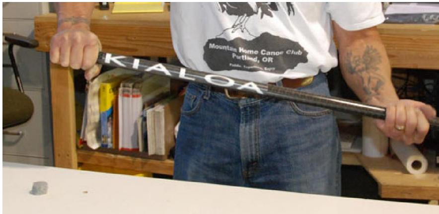
Gripping the sandpaper (around 80 grit is perfect) in your hand covering about  $\frac{3}{4}$ " of shaft and using a twisting motion with other hand, turning the shaft, is an easy way to get a good scuffing.
