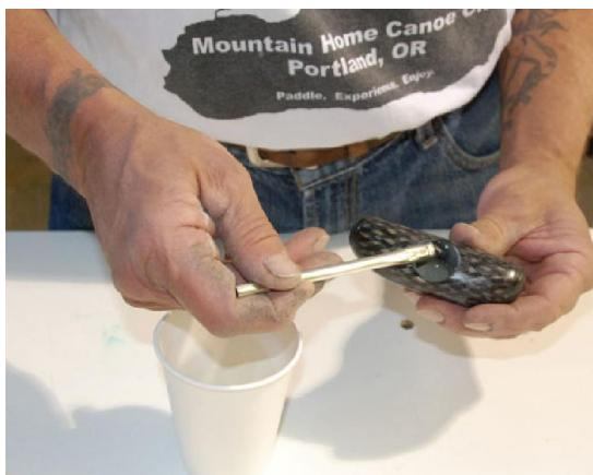
Coat the inside of the t-top as well as the sanded portion of the shaft to be inserted into the t-top and coat top of foam plug.
