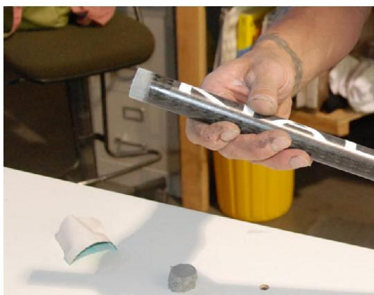
3. Insert the foam plug provided into the end of the shaft until flush with the top. This prevents glue from dripping down into the shaft and helps create a good seal.
